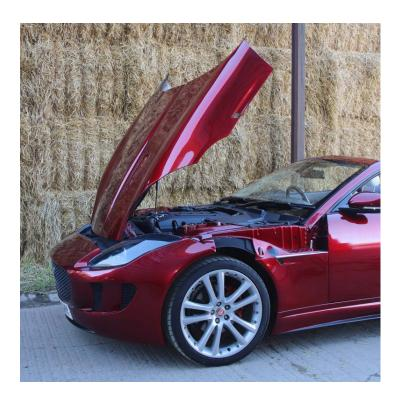
"The old front wings are removed completely," he explains. "A new lower section of wing is fitted and the top is now part of the bonnet. The wings and side skirts now flair out like the rear of the car, giving it a sexy-looking waist."
